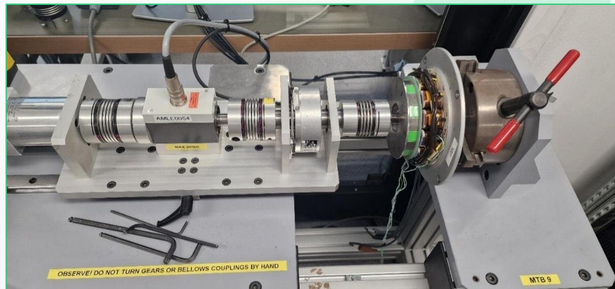
Fig 2. Highly sensitive cogging torque test-bench
