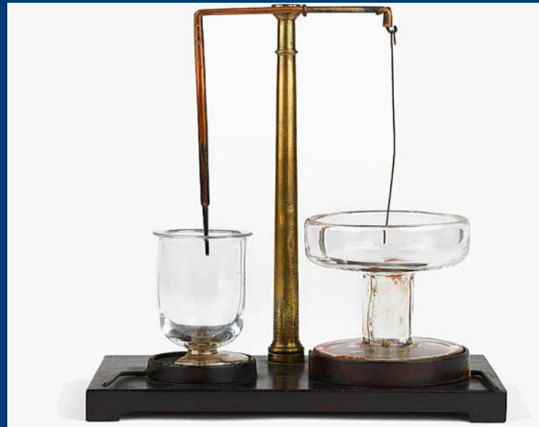
Latter Model of Faraday's "Axial Flux Motor"
