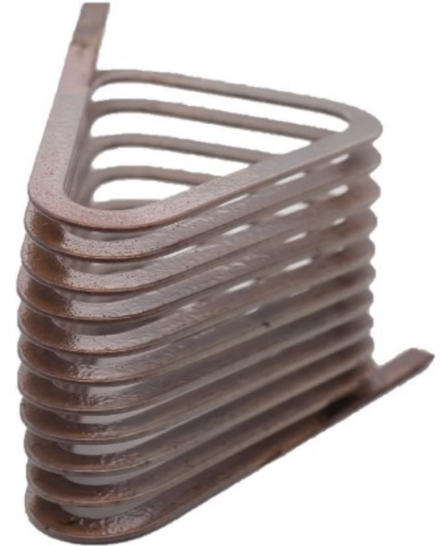
Copper coil after melting with uniform coating layer
