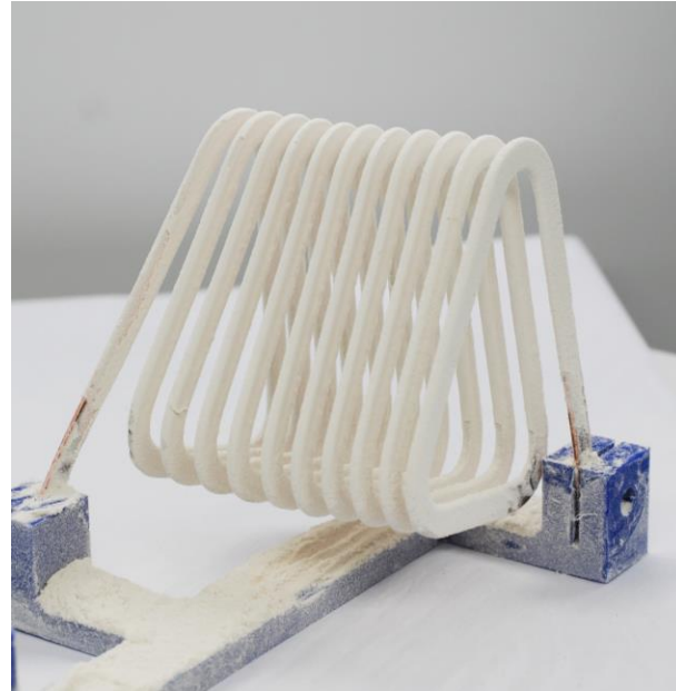
Copper coil before and after electrostatic powder coating with PEEK
