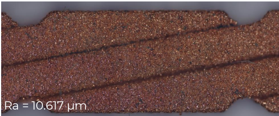
Light microscopy images before and after electropolishing
