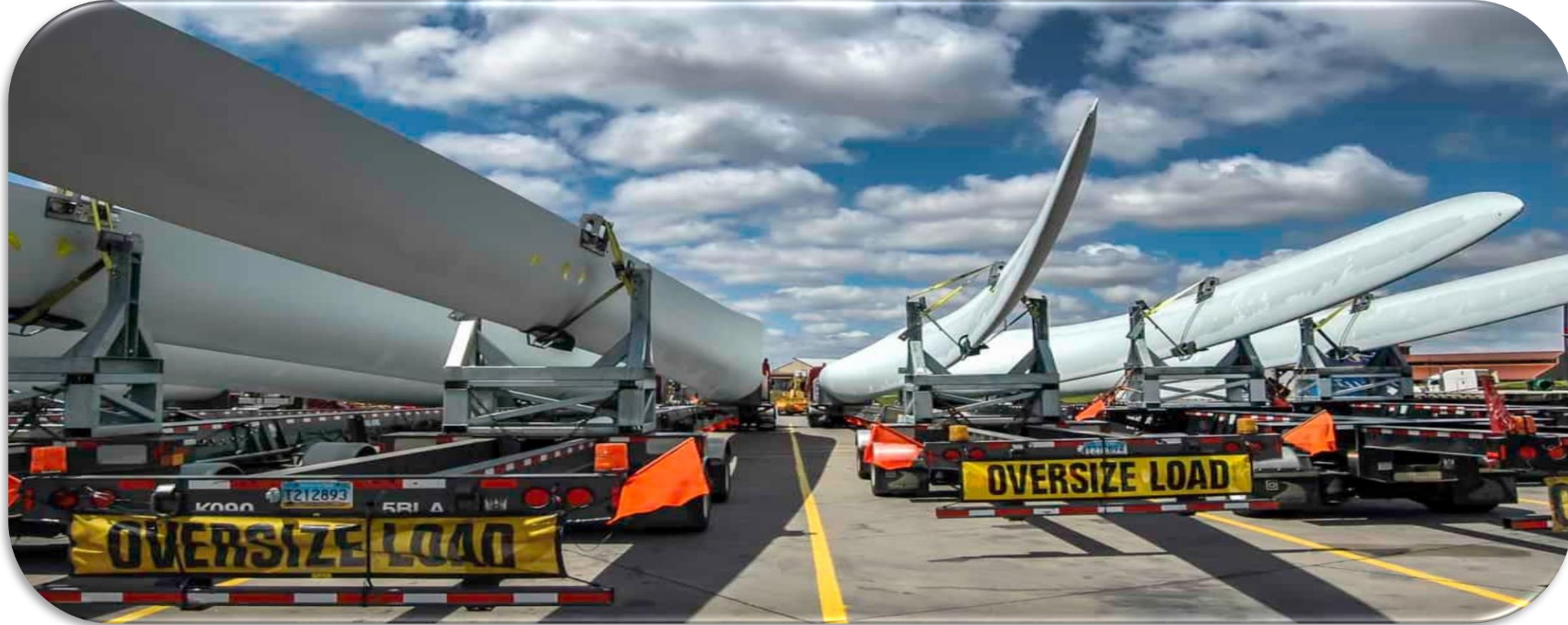
Figure 1. Oversized Wind turbine blades on semi-trucks
