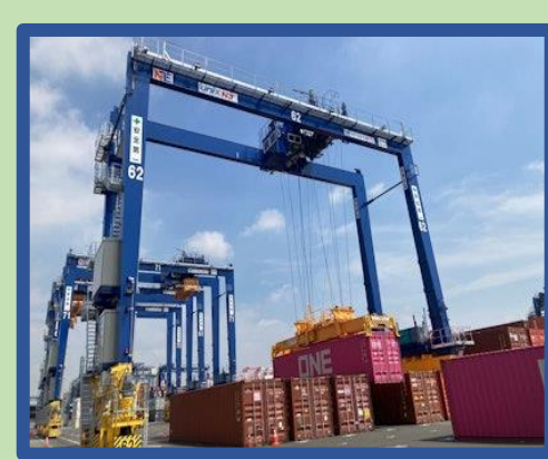
Figure 3: H2-ZE RTG Transtainer Crane
