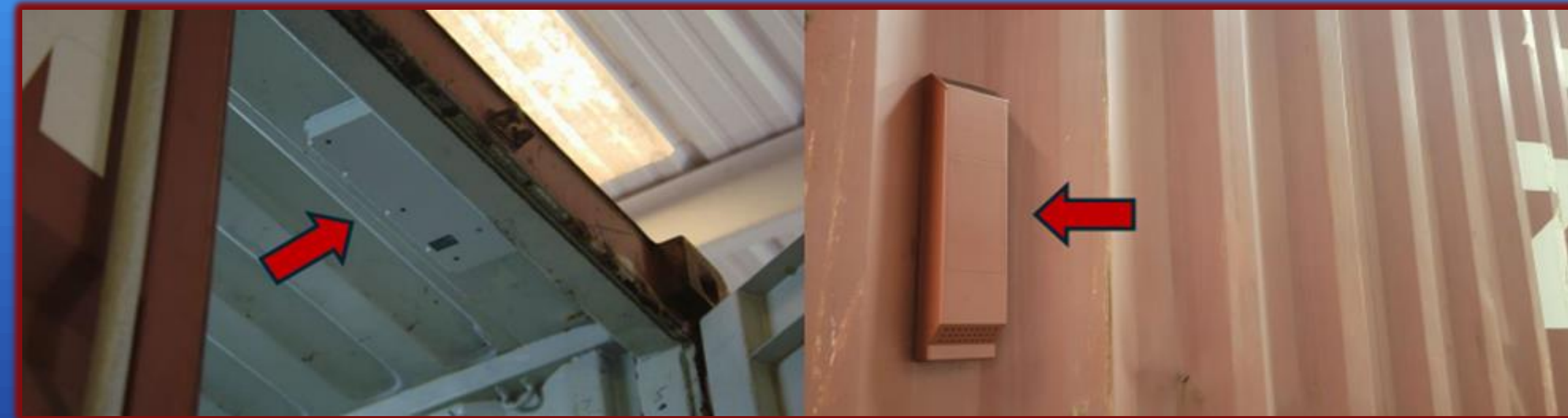
Figure 2: Image of Bloodhound's GPS technology unit looks like a container vent and is always painted to match the carriers' selected colors.
