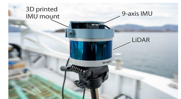
Figure 2: Lidar combined with Wit Motion 9-Axis Sensor (adapted from Sawada & Hirata, 2023)
