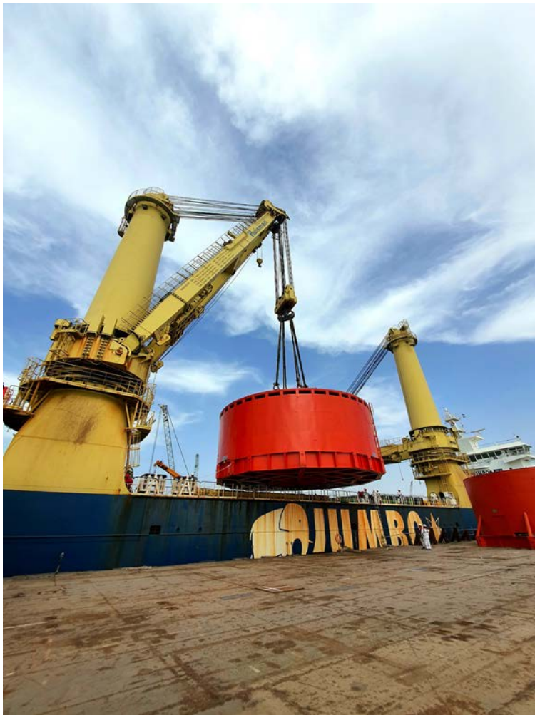
(Sixth place) Marizon Marine Services 1100 MT cable carousel offloading onto cargo barge in Abu Dhabi
